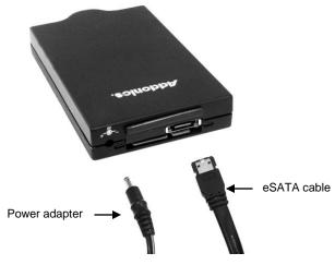
**Step 1:** Connect the eSATA cable to the eSATA port at the back of the enclosure. The other end of the cable connects to an eSATA host controller.
